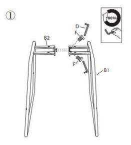
Join Stool Legs (B1) and (B2) With Bolts (F) and By using Allen Key (D) Screw to 80%
