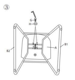
Attach Stool Seat (A) to constructed Base with Bolt (G) and Spacer (H) Using Allen Key (D)
