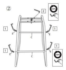
Join Connector bars (C) with Bolts(E) By using Allen Key (D) Screw to 100%, Tighten the Step ① to 100%
